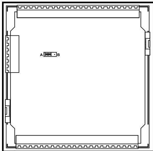
In this figure, the jumper settings will cause the inputs to function as pnp.
