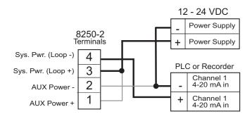
Note: **AUXILIARY power** is required to operate the relays.
