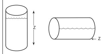
For most vessels, the zero reference point may be designated as any height in the vessel.
