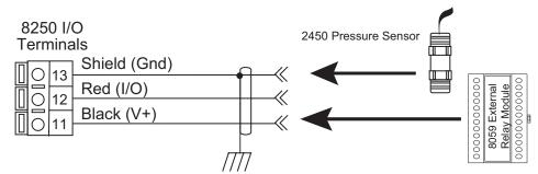
The TOTAL cable length connected to the 8250 input/output terminals must not exceed 122 m (400 ft.)
