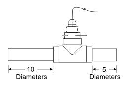
In the larger sizes, the length provided is less than ten diameters upstream and five downstream. It is not advisable to connect directly to the end of these fittings with a flow-disturbing device such as a valve or elbow. If possible, straight pipe should be added to these fittings.
