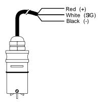
**K-factor.** If the IP80 Series meter is ordered with its fitting, the meter is factory calibrated in the fitting. A K-factor (meter factor) is indicated on the side of the fitting. This represents the actual number of pulses per gallon the meter produced during the factory flow test. This number can entered into an FT415/420 or FT5210 flow indicator to make it read properly. If a pulse divider is being used, the K-factor is the starting point for calculating the divider number.
