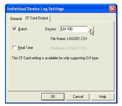
Select a trigger device in the [Device] box. This setting indicates that all logging data in the HG internal memory is copied to the CF card when the selected device turns from OFF to ON. If the selected device turns from OFF to ON again, the data in the CF card will be overwritten. In this case, enter "LM 100".
