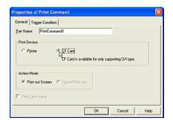
Select a [Print Device]. In this case, select "CF Card" because you will save the screen image to the CF card. The saved data in the CF card.
