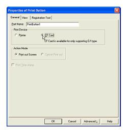
Select a [Print Device]. In this case, select "CF Card" because you will save the screen image to the CF card. The saved data in the CF card is saved as a BMP file named "CAP###.BMP". ### is a number from 001 to 009 and it is created automatically in order of the time the file was created.
