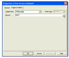
Set the Trigger Condition. For more information see "Setting a Trigger Condition" - "Executing the Command According to the State of the Device" on page 2-28. In this case, select "Falling-edge" in [Trigger Type] and enter "LM 0" to [Device].
