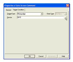
Set the Trigger Condition. For more information see "Setting a Trigger Condition" - "Executing the Command According to the State of the Device" on page 2-28. In this case, select "Rising-edge" in [Trigger Type] and enter "LM 0" as the [Device].
