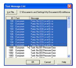
Select the text that you want to register to the project data from the list. To select multiple devices, hold down the SHIFT key or the CTRL key, and then click the text you want. In this case, select from "100" to "109".
