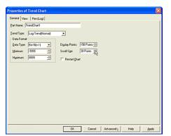
Enter a number in the [Display Points] box. This setting refers to how many a points are displayed on this object. In this case, enter "150".
