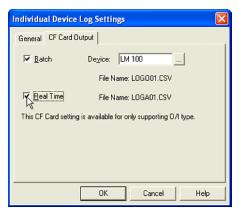
Click [Real Time] because you will copy the trend logging data when the specified sampling is done. The file name will appear in [File Name]. The copied data in the CF card is saved as a CSV file named "LOGA01.CSV". The number in the file name is the same as the Device Log No. The latest data will be added to the copied data in the CF card whenever each event occurs.
