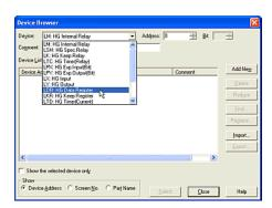
Select a [Device]. In this case, "LDR: HG Data Register".
