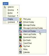
Click the [Alarm List Display] button on the toolbar (or select [Draw] [Display] [Alarm List Display] from the menu).
