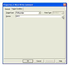
Set the Trigger Condition. For more information see "Setting a Trigger Condition" - "Executing the Command According to the State of the Device" on page 2-28. In this case, select "Falling-edge" in [Trigger Type] and enter "LM 0" as the [Device].
