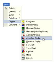
Click the [Alarm Log Display] button on the toolbar (or select [Draw] [Display] [Alarm Log Display] from the menu).
