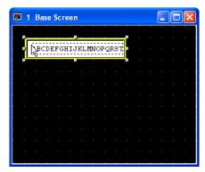
Double-click the selected object after placing on the screen. The properties dialog box will appear.
