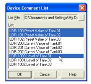
Select devices that you want to register to the project data in the [List]. To select multiple devices hold down the SHIFT key or the CTRL key, and then click the devices you want. In this case, select "LDR 100", "LDR 101" and "LDR 1000".
