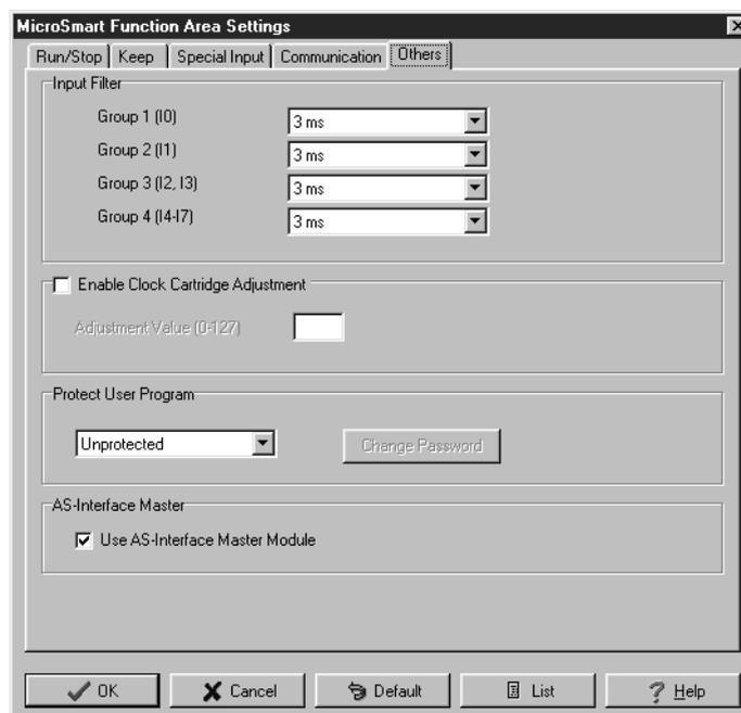
3. Make sure of a check mark in the check box on the left of **Use AS-Interface Master Module**.
