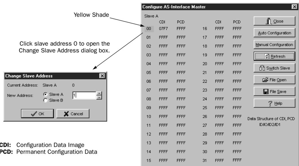
The new address “01” is shaded with yellow to indicate that the address assignment is complete.
