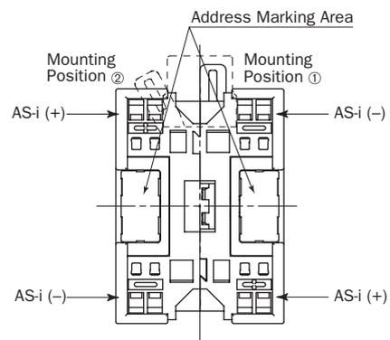
On 3-position selector, key selector, and illuminated selector switches, communication blocks ① and ② are mounted in positions shown above.
