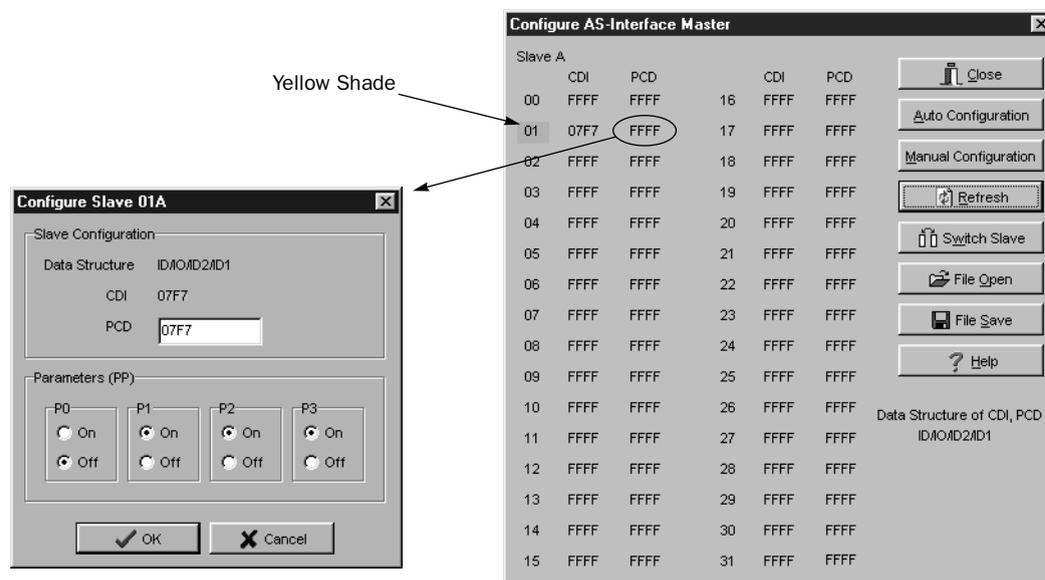
5. Click the **Manual Configuration** button to store the selected PCD and parameter values to the master module.
