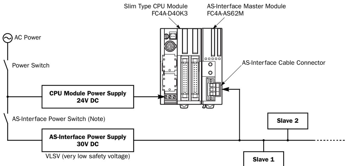
**Note:** A failed slave can be replaced with a new slave with address 0 without turning off the power to the CPU module and the AS-Interface line. But, if power has been turned off before replacing the slaves, install a new slave with address 0 and take one of the following steps, because the AS-Interface master module has to be initialized to enable communication.
