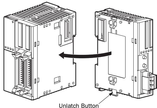
**Note:** When assembling other I/O modules with the AS-Interface master module, take the same procedure.
