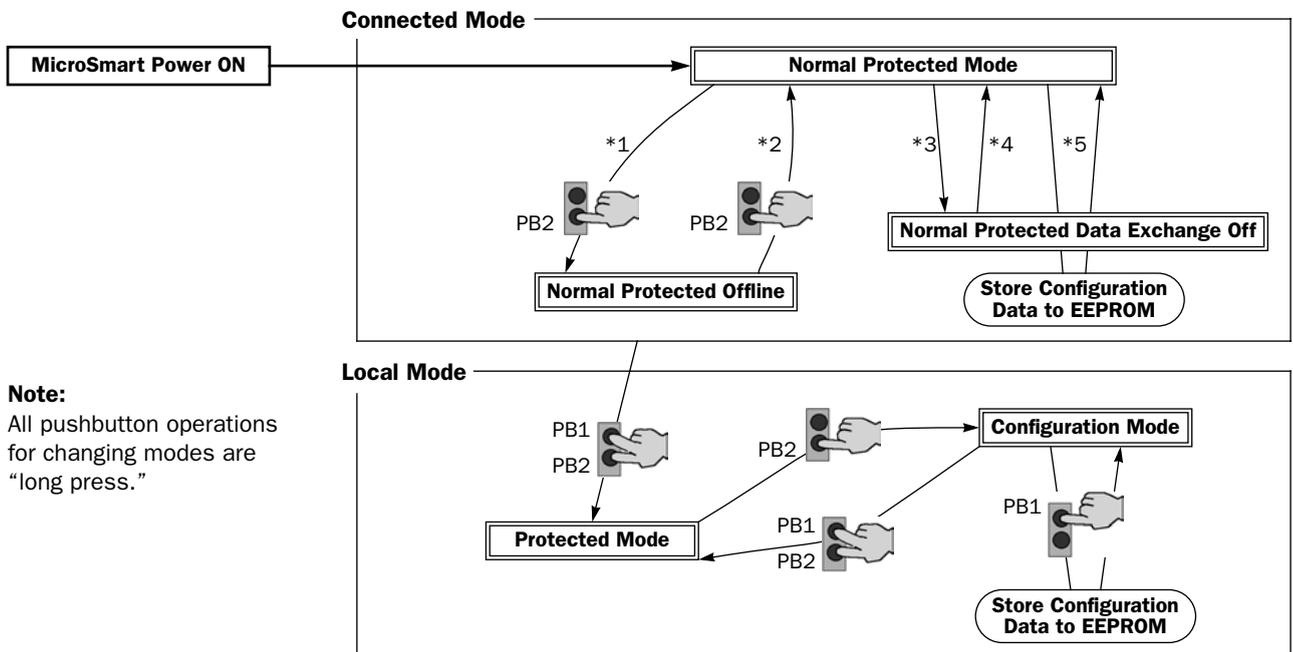
\*1 Pushbutton operation or execution of the ASI command Go to Normal Protected Offline.
