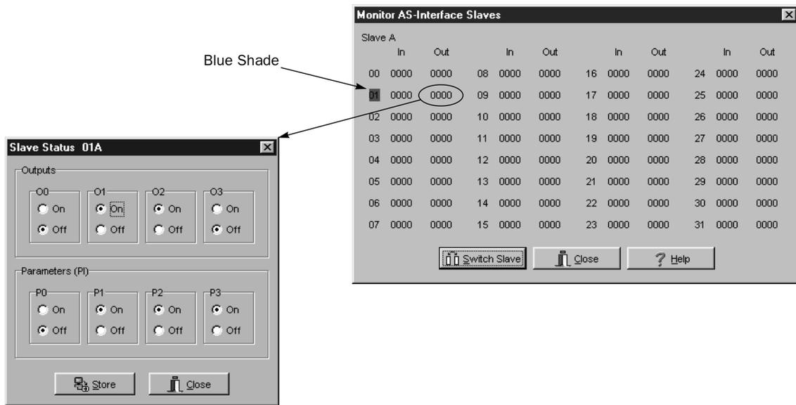
The selected parameters (PI) are in effect until the CPU module is shut down. When the CPU module is powered up again, the parameter values (PP) selected in the slave configuration procedure (page 4-4) will take effect. To store the changed parameter values to the AS-Interface master module EEPROM, execute the Copy PI to PP command by storing 0306, 0100, 0000, 0000, 0001 to data registers D1941 through D1945. See page 6-17.
