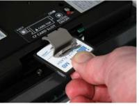
OI Touchscreens (excluding 4.6" HG1F) support Compact Flash (CF) Cards with up to 512 MB of memory. In addition to storing recipe, alarm and trending data, the CF Card can also store screen captures in a BMP format for documentation purposes. The CF Card can hold one or more projects and you can easily transfer a project directly to another touchscreen by simply inserting the card into the second touchscreen and downloading what you need.
