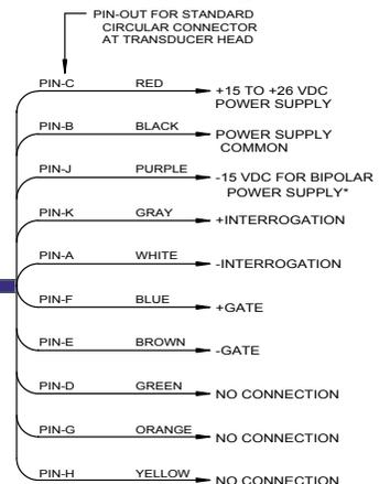
\* FOR UNIPOLAR POWER SUPPLY, IT IS RECOMMENDED TO CONNECT THIS WIRE TO POWER SUPPLY COMMON
