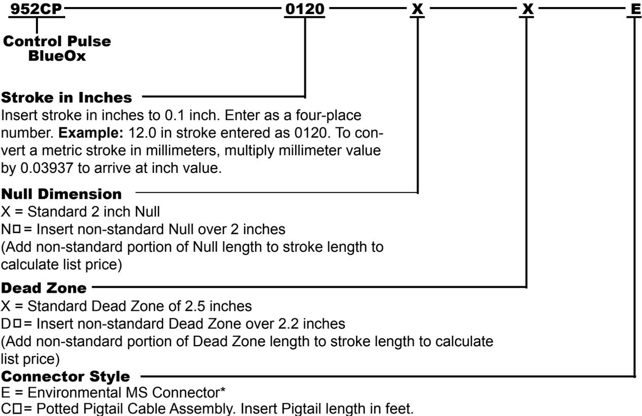
\* If option E (environmental connector) is selected, mating connector and/or pigtail must be ordered separately. **Note 1:** On unsupported stroke lengths greater than 4 feet, rod support bracket(s) and a special magnet should be used. **Note 2:** Specify magnet as separate line item (standard magnet is SD0400800).
