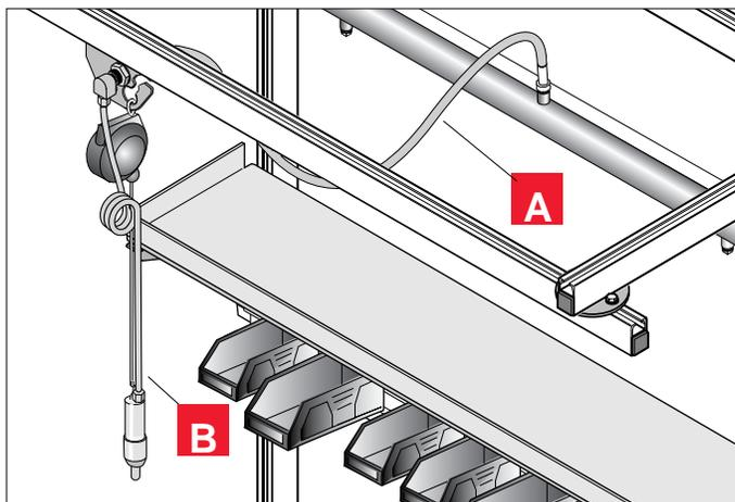
**A** The most flexible air line we have found. Ideal for connecting tool trolley to manifold or other supply because its flexibility does not interfere with trolley movement. Clear, reinforced plastic, 3/8" I.D. with 3/8" NPT male swivel fittings on both ends.
