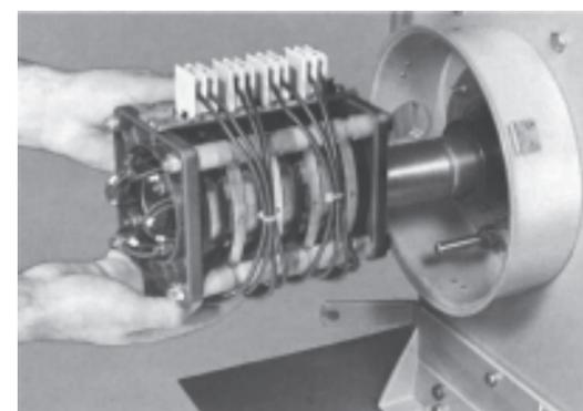
**QUICK, ONE PIECE REMOVAL...** The entire slip ring assembly can be replaced as a unit, if necessary. No need to handle small parts. To remove, simply disconnect wiring and loosen two set screws on the shaft-locking collar.
