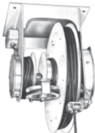
Gleason WB Reels are continuous contact reels ideal for use in applications where slip ring assemblies are not desired. No slip rings or other sliding contacts are used. Rather, a dual spool and pulley system safely and efficiently pays out and rewinds the cable.
