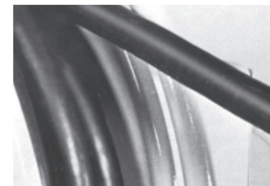
**EVEN WINDING IN MULTIPLE LAYERS...** Edges of steel flanges on cable spool are die-formed to eliminate cable pileup in corners. Segmenting of inner drum permits adjustability to suit various cable diameters – a slight change in cable size may be accommodated by the same reel with only minor field adjustment.
