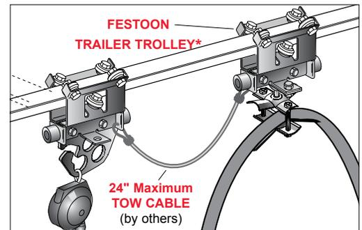
\* **FESTOON TRAILER TROLLEY** (right, bottom) provides easy management of cord or hose supplying power to tool. Fits cable or hose 0.60–0.94" (15–24mm) diameter. Tow cable connecting tool trolley to trailer trolley should not exceed 24" in length.
