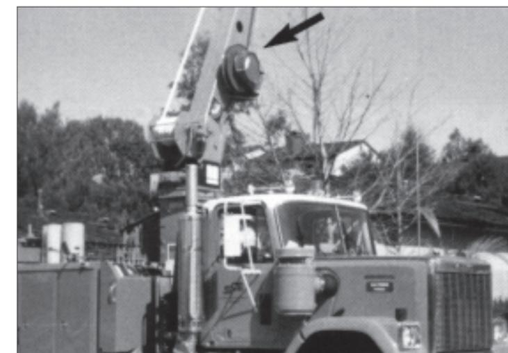
GLEASON K-REEL installed on a hoist.
