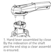
Closing torque for hand lever connection 15 Nm
