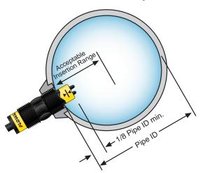
When using any type of fitting, the orientation as well as the insertion depth of the flow switch in the pipe is critical. See the diagram below for the recommended orientation depth.
