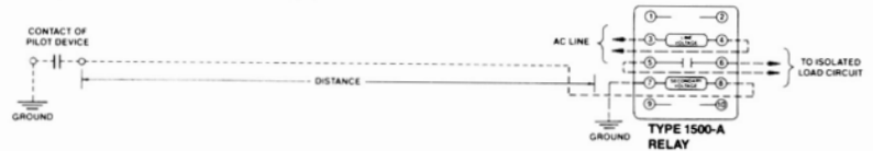
Single conductor remote control using ground return.
