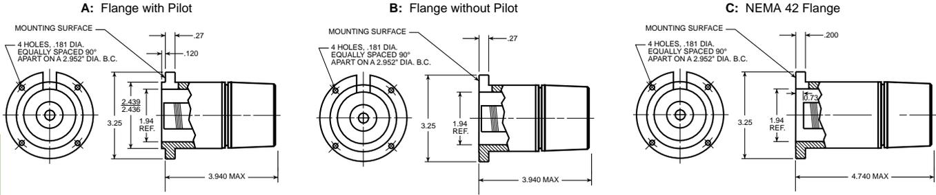
Mating shaft lengths: Typically: 0.5" max. available into the coupling as measured from the A/B mounting surface.
