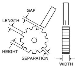
Remember to rotate the pickup so that the line on the side is parallel to gear travel.
