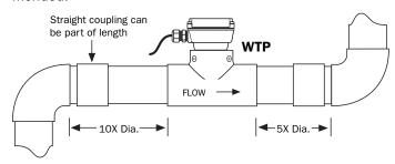
**Flanges.** For 3-8" WTC and WTS meters, standard flanges are 150 lb. ANSI drilling. 2" WTC or WTS meters and all PVC meters can be installed with optional flanges according to pipe manufacturer's recommendations. For PVC a bolt torque of 10-20 ft-lbs. for 2" flanges, 20-30 ft-lbs. for 3" and 4" flanges, and 35-50 ft-lbs. for 6" flanges is recommended.
