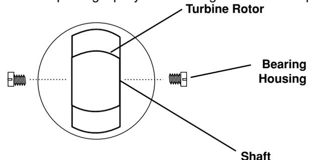
*\* Note that on ceramic shaft models the shafts are in the screws and the bearings are in the rotor. Follow the same basic procedure above. (#25945)*
