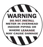
**Caution:** These water meters are not recommended for installation in uninsulated suspended ceilings where freezing is possible, or in any overhead indoor piping configuration where leakage may cause damage.
