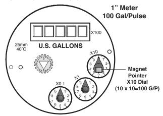
**Reading Your Meter.** The Total Flow that has passed through your meter is read by starting at the top of the register with the Five-Digit Totalizer, and then reading clockwise around the small dials. In the example below, the Five-Digit Totalizer reads  $13,800 (138 \times 100)$ , and the dials read  $60 (6 \times 10)$ ,  $2 (2 \times 1)$ , and  $.4 (4 \times .01)$  respectively. The Total Flow is 13.862.4.
