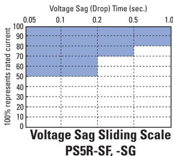
The SEMI F47 (Semiconductor Processing Equipment Voltage Sag Immunity) defines the minimum voltage sag ride-through requirements for semiconductor processing, automated test equipment, and other equipment. It requires that the equipment be able to tolerate voltage sags on an AC power line without interrupting operations. This avoids the loss of production and money.
