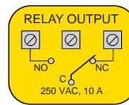
The relay is a single pole, double throw type rated at 250 Volts AC, 10 Amps. The two terminal NO and NC (normally open and normally closed) will be used in different applications. Remember that the "normal" state is when the relay coil is de-energized and the Red relay LED is Off / de-energized.
