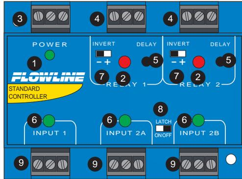
1. **Power indicator:** This green LED lights when AC power is ON.
