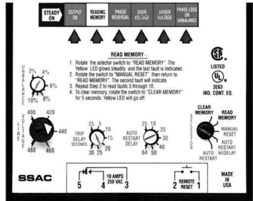
**Manual Reset (Onboard):** Rotate selector switch from the Manual Reset position to Auto Restart w/ Delay then back again to Manual Reset within 3 seconds. The output will immediately energize.
