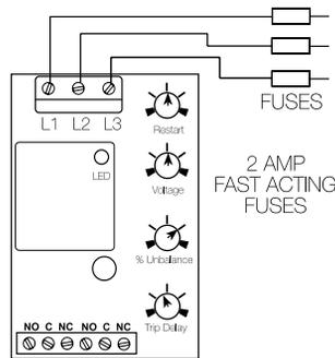
**CAUTION:** 2 amp max. fast acting fuses are recommended to protect the equipment's wiring. They are not required to protect the HLMU.
