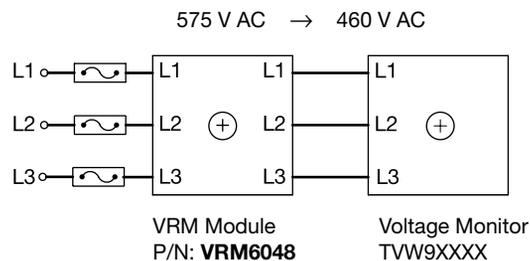
\* The VRM6048 must be connected as shown. If the TVW9XXX is disconnected, the VRM output voltage equals the input voltage.
