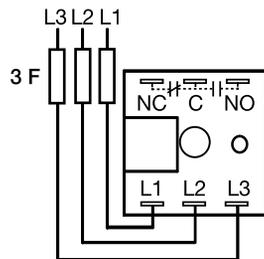
Relay contacts are isolated. Dashed lines are internal connections.
