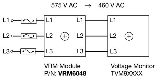
\* The VRM6048 must be connected as shown. If the TVM9XXX is disconnected, the VRM output voltage equals the input voltage.
