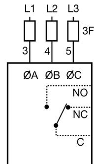
2 Amp Fast Acting Fuses Recommended For Safety (Not Required)
